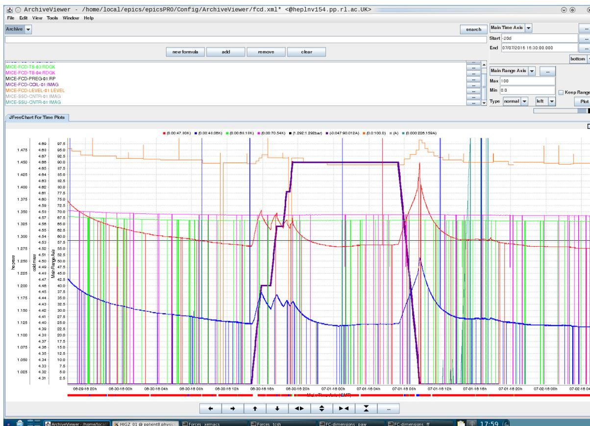
Figure 2 Archive Viewer traces of a ramp up and down of FCD. Red line = cold mass temperature (TS01); blue line = He bath temperature (TS02); thick purple line = current (up to 90 Amperes).
