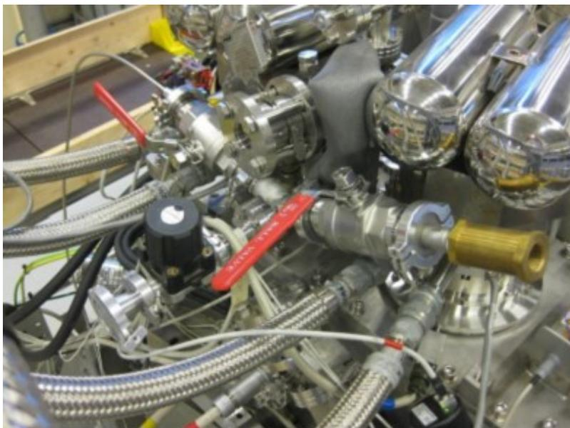
Figure 3 Helium supply valve (red handle on the left) and pressure relief valve (right) of the FC. The supply valve is open when the red handle is in line with the He supply pipe, as shown.
