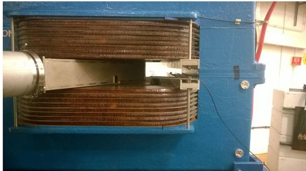
**Figure 1:** Bending dipole D1
