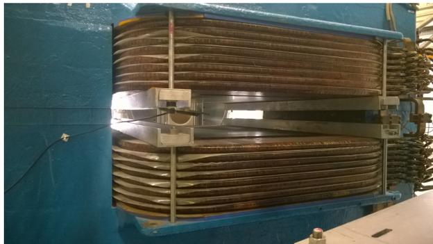
**Figure 2:** Bending dipole D2
