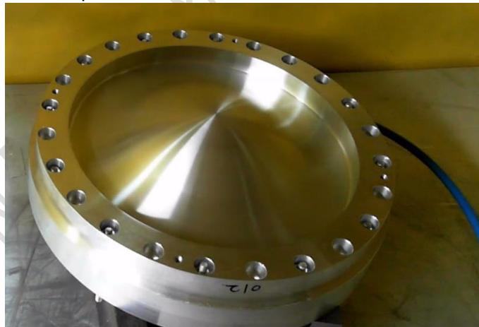
Window Test assembly in chamber prior to test
