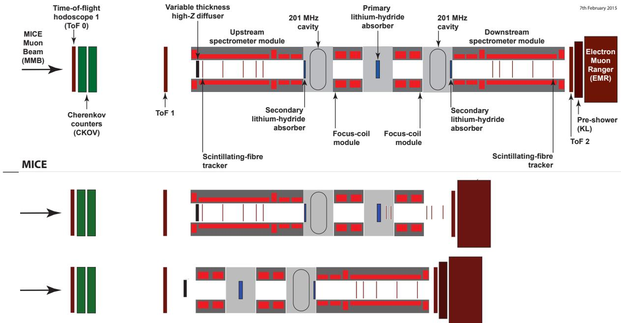
Figure 3: Top: schematic diagram of the cooling-demonstration configuration. Centre and bottom: schematics of the descope options discussed in the text that may be considered in the event that the downstream solenoid is not available.
