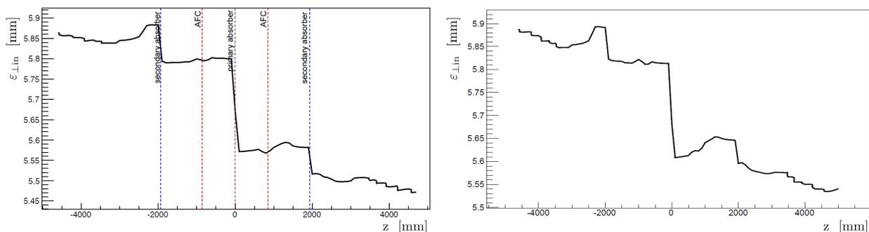
Figure 2: Emittance reduction with (left) two high-power RF amplifier (baseline condition) and (right) with only one RF amplifier available.
