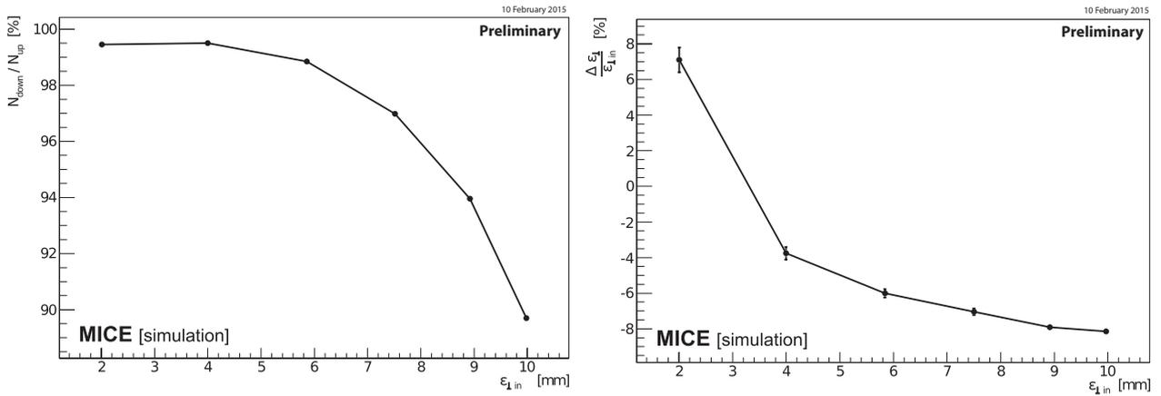
Figure 1: Transmission (left) and emittance reduction (right) as a function of input emittance for 200 MeV/c beams. The error bars correspond to  $\sim 100k$  muons passing through the experiment.
