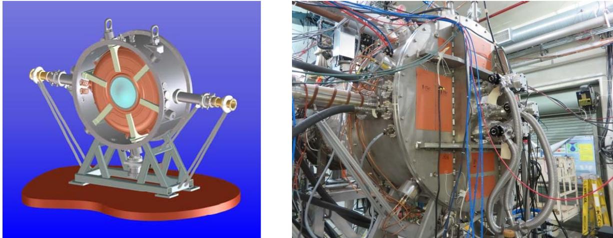
*Figure 4: 3D model showing main features of the cavity and SCTS, this will also be the model for the cavity sections of the IC experiment. Photograph of the instrumented cavity in the MTA*
