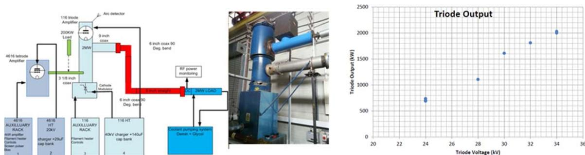
*Figure 2: Showing the layout of the test station at Daresbury, an image of the final stage amplifier and the variation of amplifier chain output power with triode valve bias voltage*
