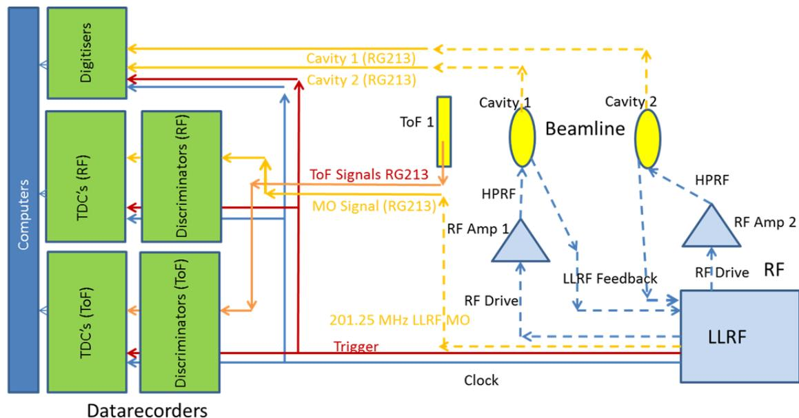
Figure 5: Overview of RF and ToF signal routes for determination of muon transit phase. Dashed lines correspond to high performance microwave cable.
