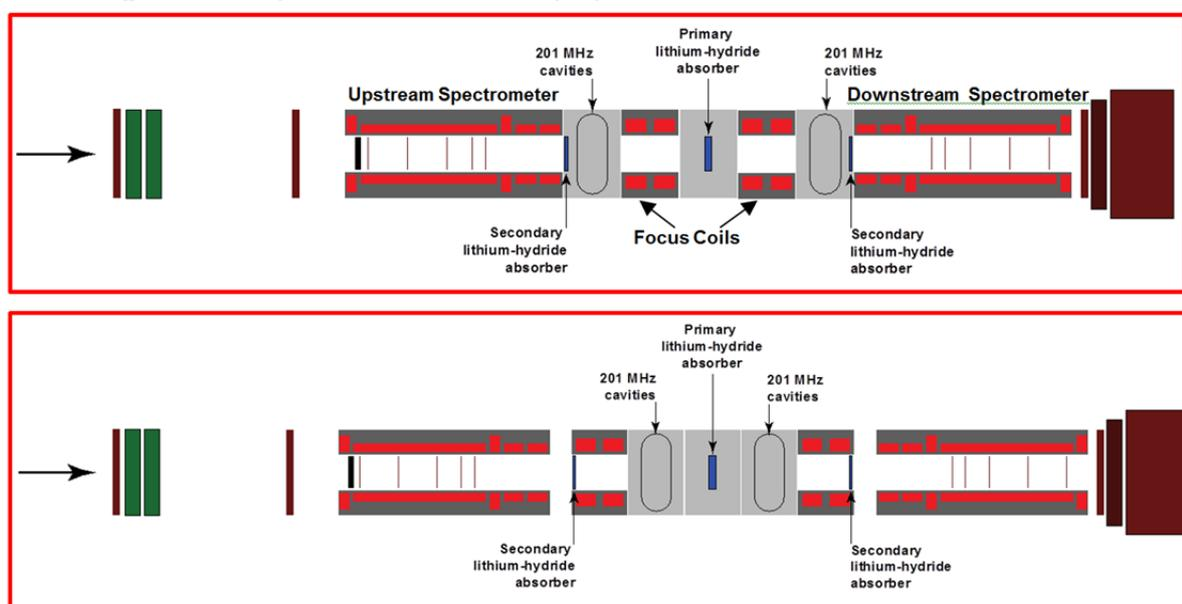
*Figure 1: The main components of the MICE Ionisation Cooling (IC) apparatus, upper figure is the reference design, lower figure is an alternative lattice being considered at the time of writing. There are no substantive differences between these from an installation and commissioning perspective.*
