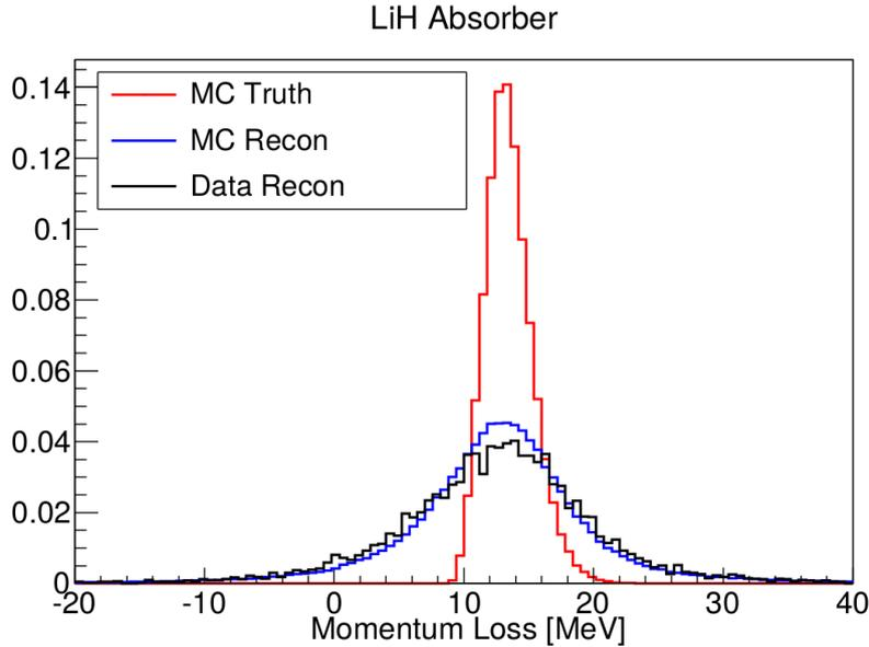
Figure 2: Measured change in momentum for a set of muons passing through the lithium-hydride absorber is shown as the black histogram. The simulated momentum-loss distribution is shown in red (“MC Truth”). The simulated momentum-loss distribution after detector and reconstruction effects have been taken into account is shown in blue (“MC Recon”).
