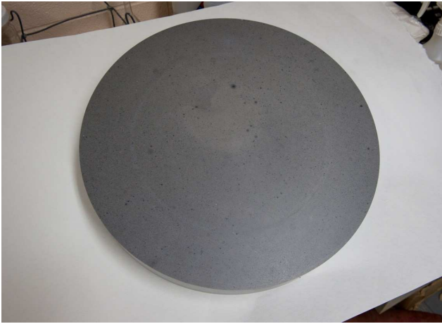
Figure 2: LiH disk absorber, complete and coated.
