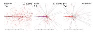
Due to the high granularity of the detector it is possible to identify each particle type and measure its range and energy:
