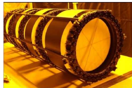
Figure 2: The MICE scintillating-fibre tracker.
